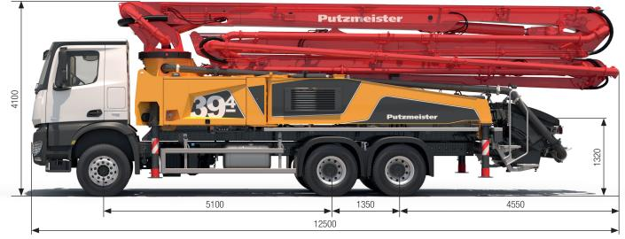
Note: Standard version. Dimensions and weights depend on truck, pump model and equipment. Dimensions in mm for MB-Arocs 3342. Illustrations show special equipment.
