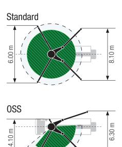
Support width based on center of support leg
